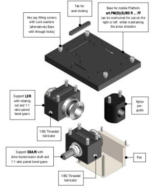
> On request it is possible to use two different special accessories on the mobile Platform of which one for play adjustment, whilst the other in vertical/oblique use has the function of indicating rotary nutwear (see page .233).
