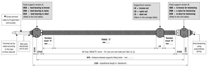
LENGTH = LB on page 65/M - CFS/A - CFS/B on page 65/O - CF/FB(x2) on page 65/P (normally the length LB is substituted with the length of the entire carriage)
