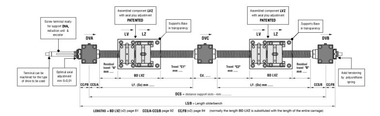
• TRAPEZOIDAL SCREW MANOEUVRING GROUP mod. "COMPACT STEEL BIDIRECTIONAL"- art.C/DVABC+LV2 ... R/L series 20/60
