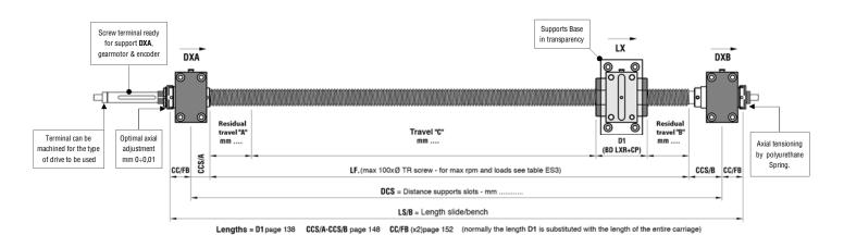
TRAPEZOIDAL SCREW DESIGN of threaded bar ready for the above supports, gearmotor (positioned at the side or above) & encoder.
