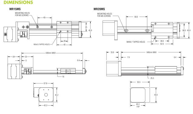
Note: Maximum length for lead screw driven MR is 640 mm.
